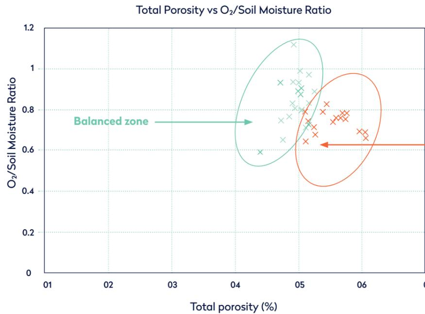
**Figure 26:** Scatter plot of measured total porosity against the O<sub>2</sub>/soil moisture ratio
